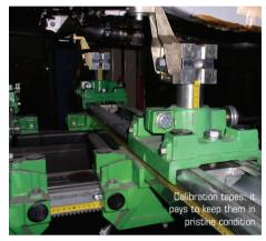
"Let's deal with the easy ones first. Users often assume that because a bracket is available, it must be secured to the vehicle, when in practice it's the extent of the damage that must dictate the number and location of brackets employed. Securing brackets unnecessarily is unproductive", says Matt.
